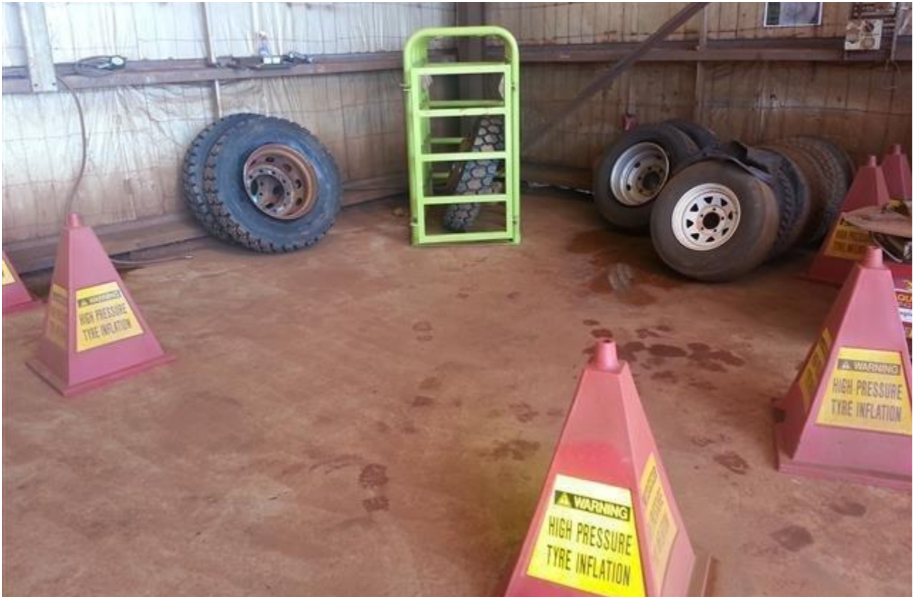
Photo of barriers with signage to inform personnel and visitors of clearance zone for tyre safety inflation cage.
