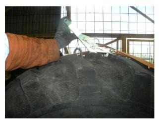
Two (2) tyre service persons were performing a change on a backhoe tyre (18.4-26) using a floor mounted tyre change machine. Whilst undertaking this task they had trouble seating the beads of the tyre to the rim. A bead blaster was used several times, to assist with the task, however this still proved unsuccessful. It was decided that a tie-down ratchet strap be used to help seat the beads. The ratchet strap was placed on the tyre and inflated and the beads seated.
